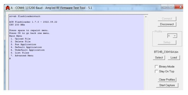
2. Use the "Upload File" option from the menu to begin loading over y-modem a new "Application/Executable" file.
