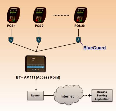
Combined with our POS adaptor (BT-POS111), the Bluetooth access point (BT-AP 111) offers ethernet conectivity for up to 20 "tether free" card readers.
